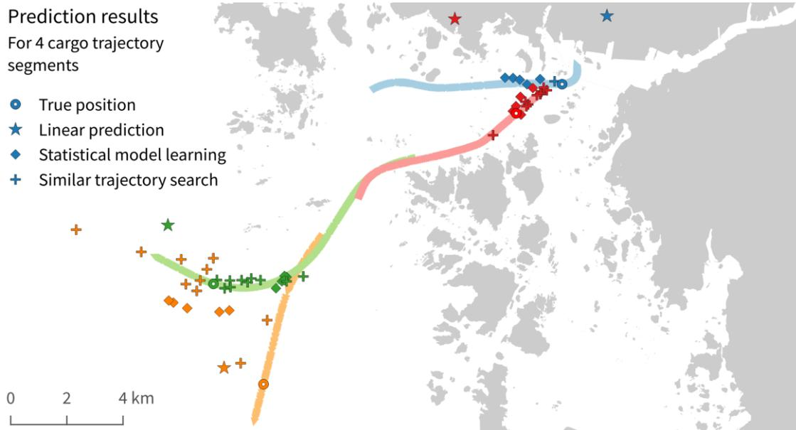
Figure 3. Predicted future locations after 15 minutes for two incoming (red and blue) and two outgoing (orange and green) cargo vessel trajectories.
