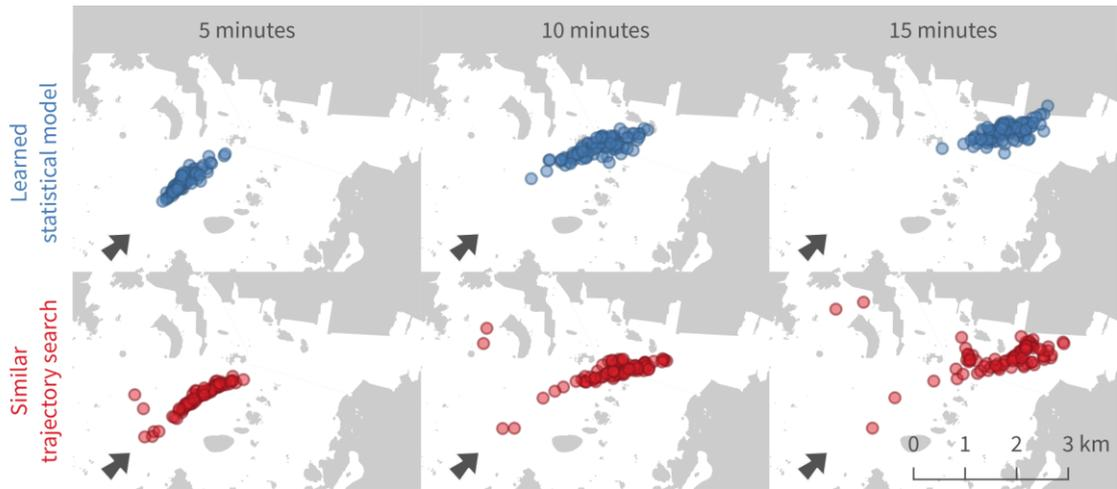
Figure 2. Potential future locations after 5/10/15 minutes based on the learned statistical model (top row, blue dots) and similar trajectory search (bottom row, red dots). Start position and heading depicted by the black arrow.
