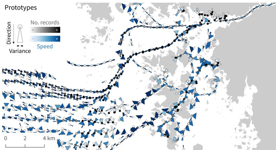
Figure 1. Learned prototypes in Gothenburg: speed (triangle colour), mean direction (triangle orientation), variability of direction values (triangle width), and number of records (circle colour). Background map data: OSM.
